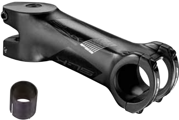
Shim to adapt 1-1/4" stem to 1-1/8" steer tube
